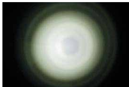
Irregular LED beam (contains rings and spots)
