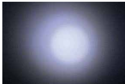
Irregular beam (brighter spot at center)
