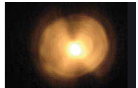
Irregular incandescent beam (contains rings and spots)
