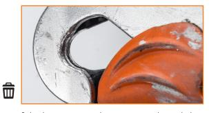
Side plate worn around connector attachment hole.
