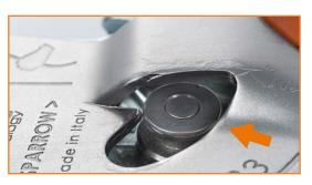
Movable side plate bent, cam pivot does not engage correctly.
