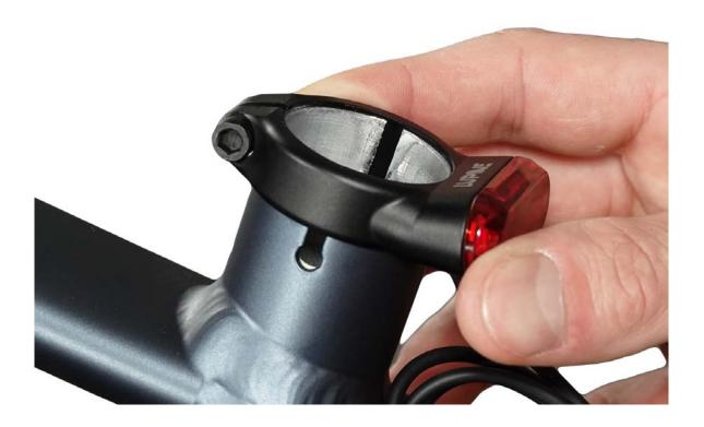
Note: The stop lip of the C14 must be flush with the seat tube.
