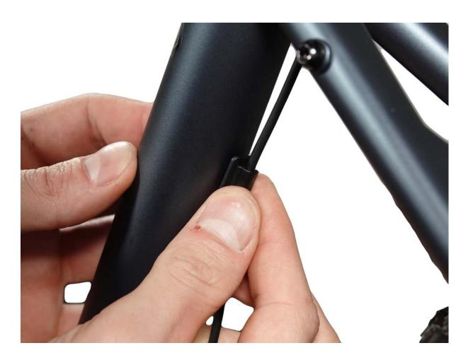
Note: In order to find the suitable locations, it is advantageous to plug the cable into the cable guide before gluing.
